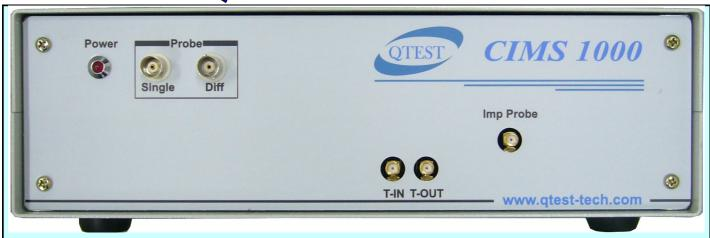
Qtest CIMS1000 is a new approach to measurement of CI or the Characteristic Impedance on printed circuit board and cables. It uses the basic components of L and C in the calculation of CI measured on a pcb or cable. Zo=Sqrt( L/C) is the basic formula in the calculation of impedance.
