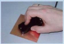
The SP-100 probe, intended for measuring thickness of copper laminate of unetched PCB, uses a four-point electrical resistance measuring principle.
