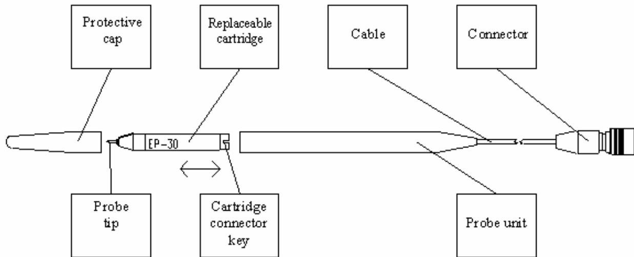
Fig. 3. Probe unit with replaceable cartridge
