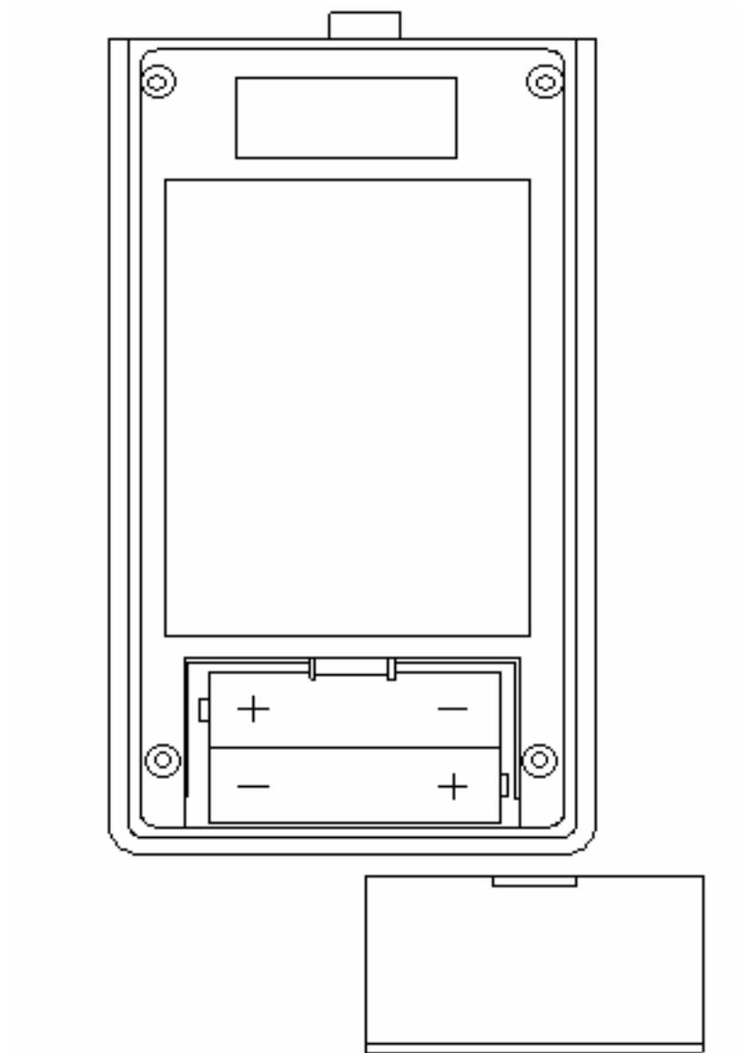
Fig.2. ITM-525. Rear view. Cover of battery compartment is open
